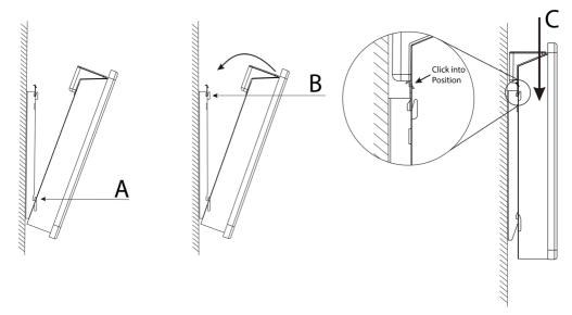
To mount the heater onto the wall, tilt the heater so the bottom holes in the rear of the heater are aimed at the lower mounting hook and attach the heater on to the bracket (A).
